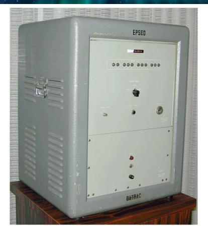
1954 "DATRAC" 11-bit, 50-kSPS Vacuum Tube ADC Designed by Bernard M. Gordon at EPSCO 500watts, 150lbs, \$8500
